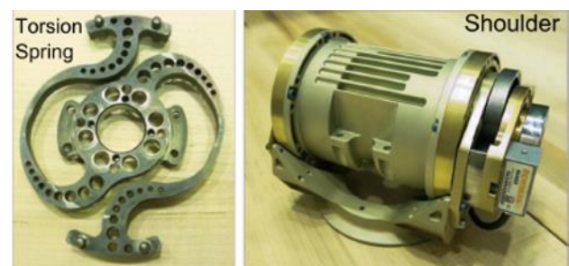
Figure 6: Left: torsion spring developed by NASA for humanoid robot Valkyrie; Right: SEA Actuator mounting the torsion spring in series to the output
